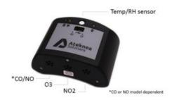
The LEO is a portable sensor pack. It measures NO, NO<sub>2</sub> and O<sub>3</sub> using electrochemical sensors. It also provides information about the current temperature and relative humidity. It can be used both, outdoors and indoors, but its primary use is for outdoors.
