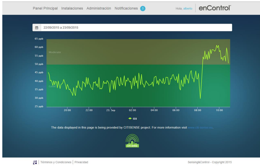
Figure 7: Ozone (O3) raw data aggregated (avg) on 5 minute interval with AQI on background.
