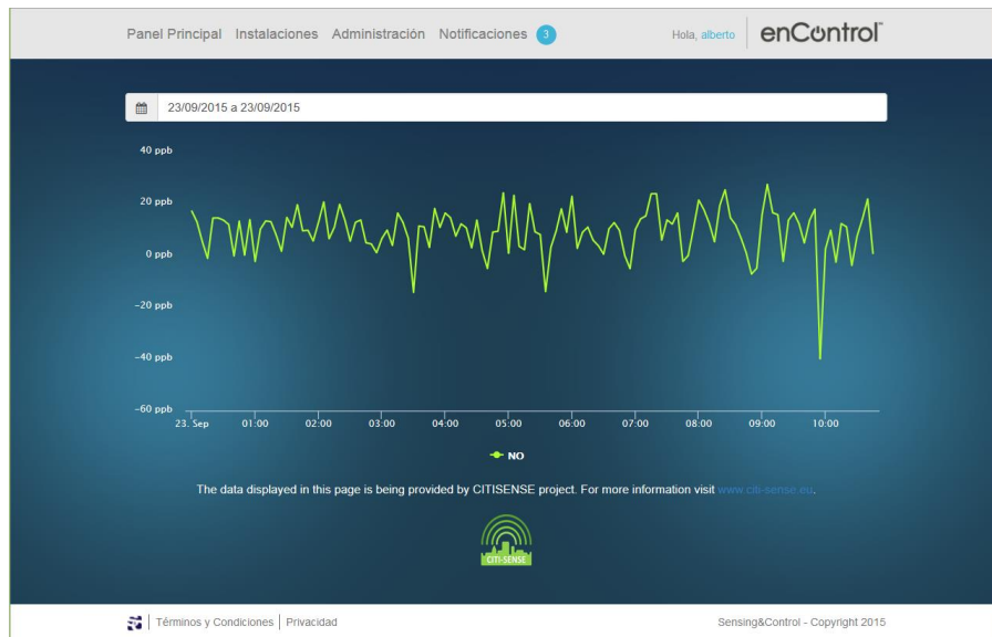
Figure 5: Nitrogen Oxide (NO) raw data aggregated (avg) on 5 minute interval
